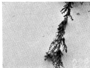
Fig. 8. Transformation of crystals of n -dotriacontane caused by the addition of the alcohol fraction of asphalt components (micro-crystallized).
